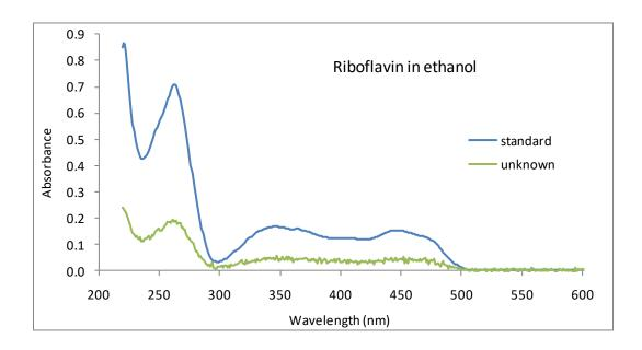
The main utility of plotting the spectral data is to check that the overall shape of the curves are the same. Additional peaks in the unknown spectrum could indicate the presence of interferences. Many substances absorb in the UV region, and in this case the strongest riboflavin absorption is near 260 nm.
