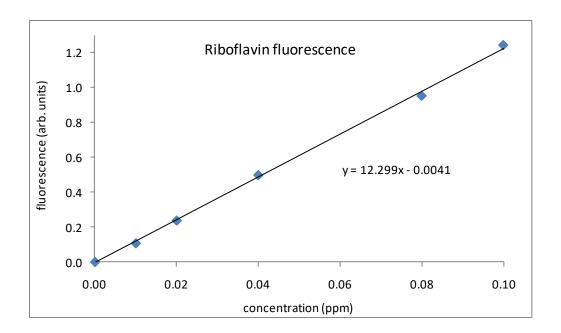
The main reason to plot the calibration data is to check that the measurement is linear over the concentration range of interest. In this case we can be sure that the instrument does respond linearly from zero to 0.10 ppm riboflavin.
